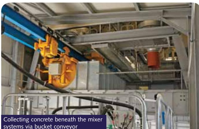
Collecting concrete beneath the mixer systems via bucket conveyor
